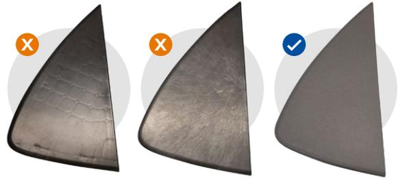
Solid part which designs for foaming process (e.g. Rib ratio, thinner wall thickness, etc.) shows all defects (sink marks etc.)
